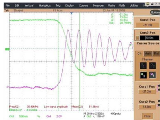
Fig. 9 - Measured Current and Voltage Turn-Off Switching Transient
