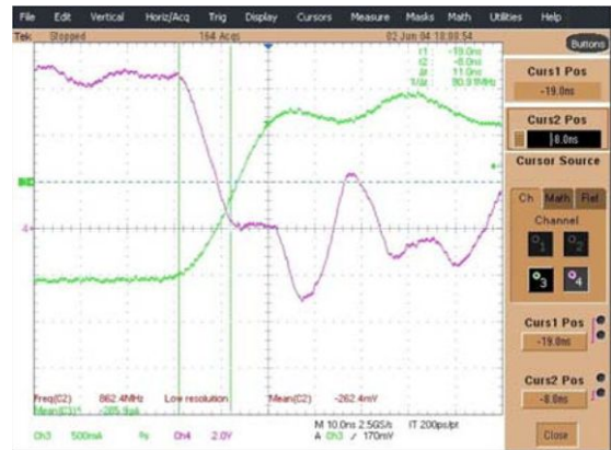
Fig. 8 - Measured Current and Voltage Turn-On Switching Transient
